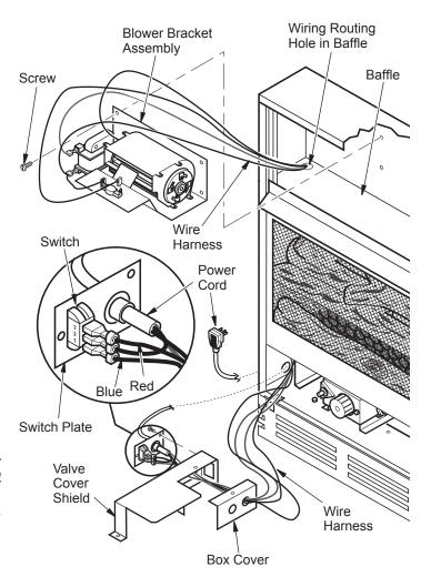
Figure 4 - Installing Blower Bracket Assembly
