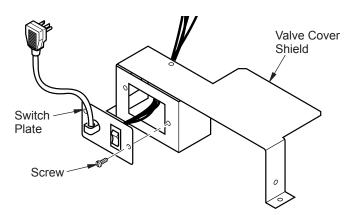
Figure 5 - Installing Switch Plate to Valve Cover Shield
