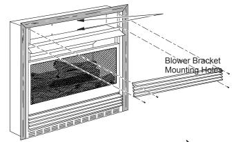
Figure 2 - Removing Upper Louver Assembly
