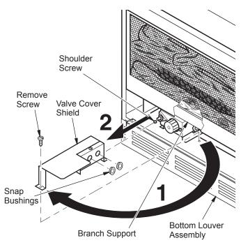
Figure 3 - Removing Valve Cover Shield
