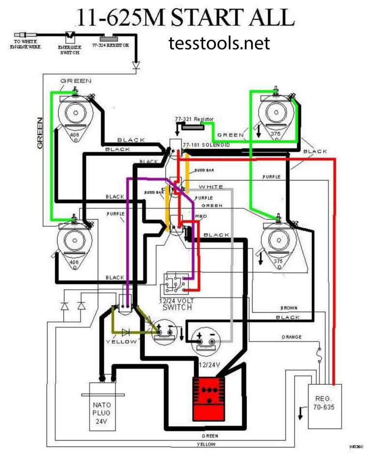
**REPLACEMENT PARTS:** 79-406 Generator isolated ground 79-375 Generator case ground 70-045 Engine pulley 79-405 Brush set for one generator 71-819 V helts 890-635 Regulator 70-441 Cable and clamp assembly with red plug 77-181 Solenoid 71-510 Voltmeter 71-520 Ammeter 890-445 12/24 switch assembly 77-321 Output resistor assembly 70-621 Energize button assembly 77-324 Energize Resistor Assembly
